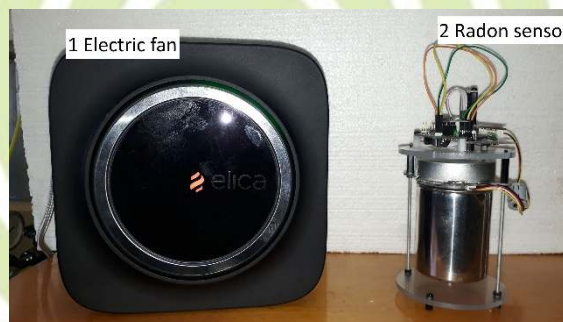
Figure 5. Photo of the Respire Monitoring and Remediation System. Electric fan for ventilation (SNAP, © Elica S.p.A.) (1) connected via Bluetooth to the radon sensor (2).
