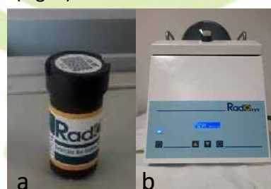
Figure 4. Radosys CR39 long-term indoor radon detector (a); automatic system for reading the alpha traces on the films of the exposed dosimeters (b).
