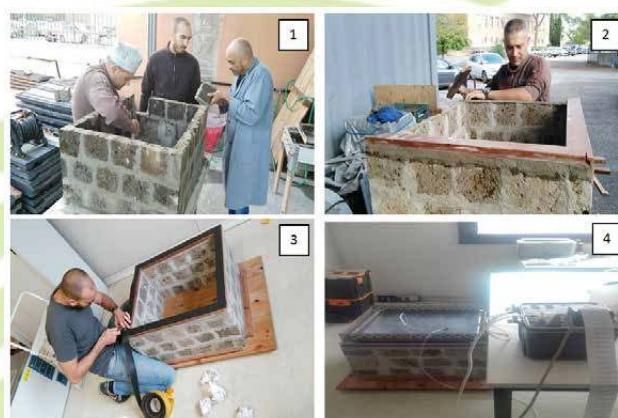
Figure 6. Construction of the model room (1,2,3) and its connection with the RAD7 detector for continuous monitoring of radon during the experiments (4).
