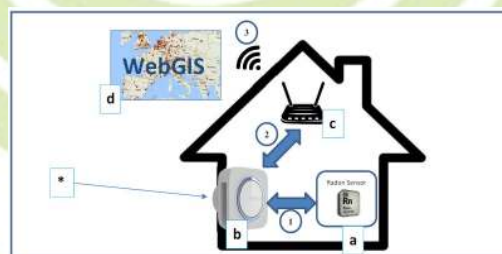
Figure 2. Scheme showing integration and communication between the various components of the prototype system. (a) Radon sensor module developed by CERi; (b) SnapRn developed by Elica S.p.a.; (c) domestic router; (d) WebGIS database; (1) RF communications; (2) WiFi (802.11 b/g/n); (3) MQTT protocol; * - Snap is equipped with a brushless motor.
