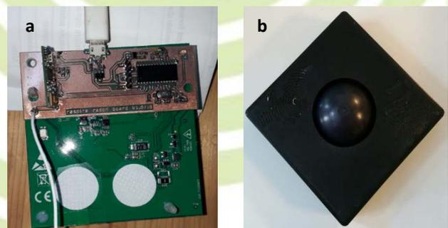
Figure 7. Interface board (29.97 x 77.47mm) (above) overlaid on the Rn sensor board (below) and linked by using a 6 pin connector (a); housing designed ad-hoc and made with a 3D printer (b).
