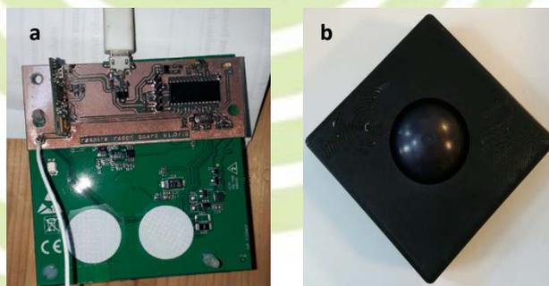
Figure 7. Interface board (29.97 x 77.47mm) (above) overlaid on the Rn sensor board (below) and linked by using a 6 pin connector (a); housing designed ad-hoc and made with a 3D printer (b).
