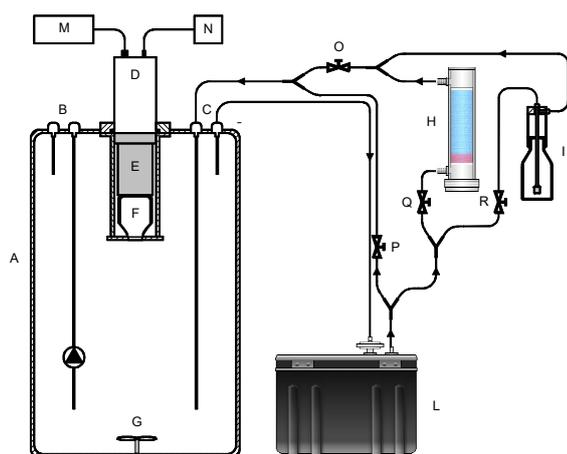
Figure 2. Experimental set-up. A) radon chamber; B) air tight connectors (CPC) to be used when air circulation needs a pump; C) air tight connectors (CPC) when air circulation is guaranteed by an outer device; D) signal processing module; E) photomultiplier; F) scintillating flask; G) fan; H) desiccant column (Drierite); I) humidifying device; L) Durridge RAD7; M) multiscaler, N) low voltage supply; O), P), Q) and R) stopcocks (De Simone *et al.*, 2016).
