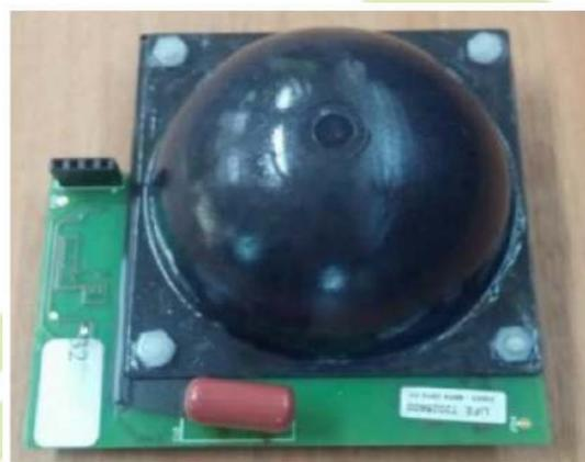
Figure 6. Radon SS Gas Sensor, 1750 pCi/l Rn EURO-GAS Management Service LTD.
